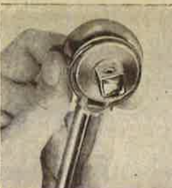
Insert unit in handle, holding cap in place. Put snap ring in position.
